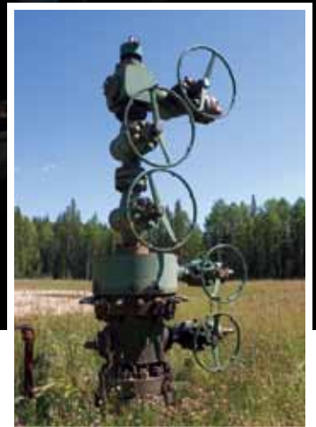
Although a pumpjack is a recognizable symbol of oil production, modern oil and gas operations — those that use horizontal drilling and fracking technologies — no longer need the pumps. After drilling (left) is complete, all that remains is a collection of valves (right), often referred to as “Christmas trees.”
